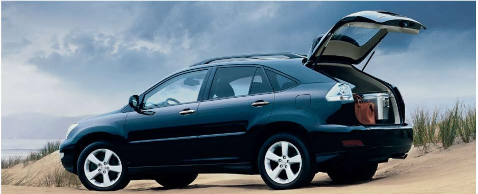
The power rear door can be raised or lowered by pressing a button on the key, inside the cabin or on the door itself. For safety purposes, a series of beeps will alert those standing nearby whenever the door function is activated. If the button is activated while cargo is being loaded, a resistance sensor will prevent the door from lowering.
